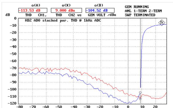
Figure 16: THD vs. level of the two input channels of the dual-range AD converter
