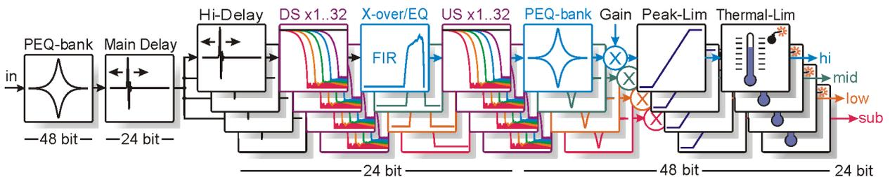
Figure 1b: Signal processing in one DSP for one input and a group of four output channels
