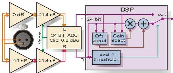
Figure 15: Dual-range AD conversion principle
