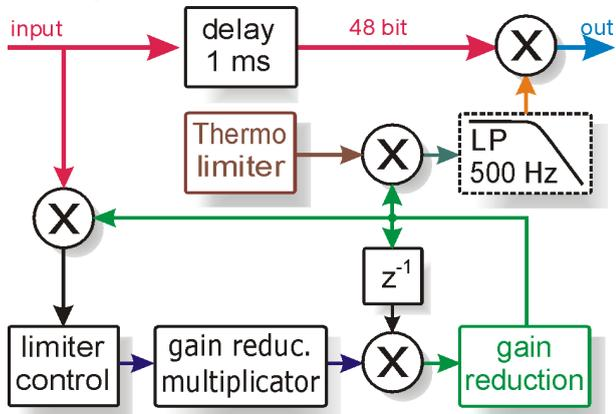
Figure 17: Block diagram of look-ahead peak limiter
