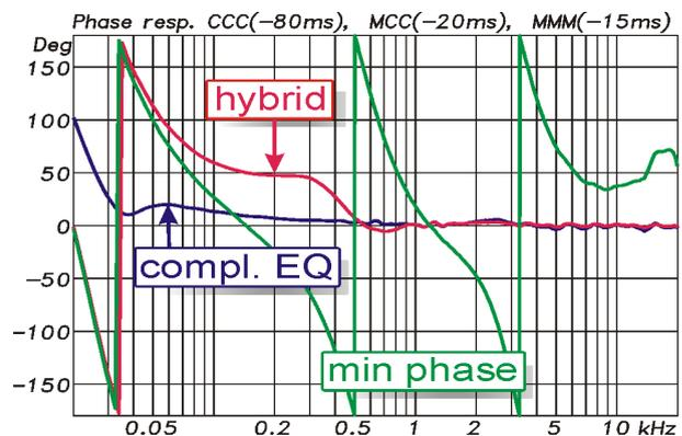
Figure 5: Phase response for complex equalization, overall minimum phase and combined minimum phase and complex equalization
