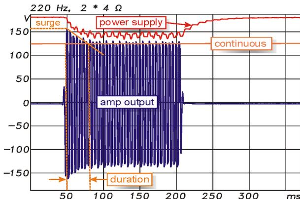
Figure 20: Determination of parameters for “controlled overshoot” limiter threshold adaptation.
