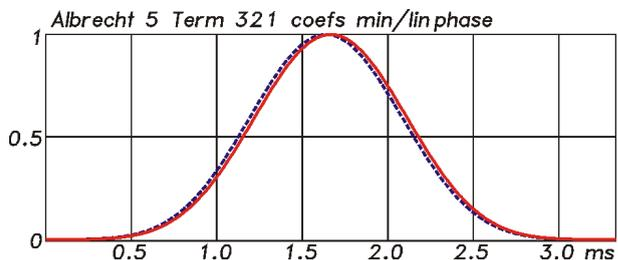
Figure 6: IR of anti-alias low-pass. Solid line: linear phase, dotted line: minimum-phase.
