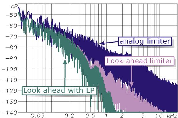
Figure 19: Gain reduction spectrum in conventional analog peak limiter compared to look-ahead limiter with and without 500 Hz low-pass.
