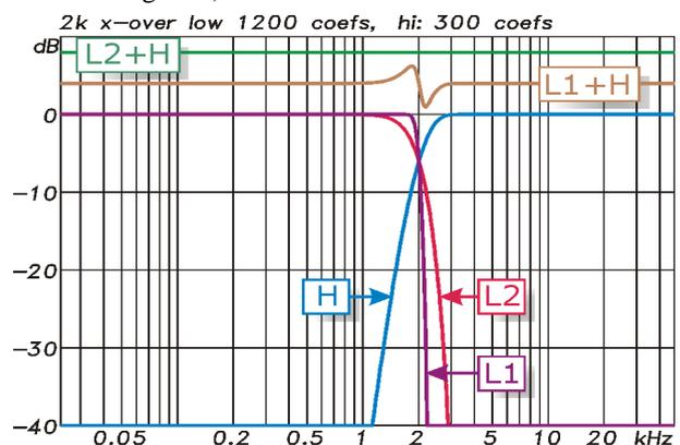
Figure 9: Effect of adding asymmetrical slopes (L1+H) and correction by pre-windowing the IR (L2+H)
