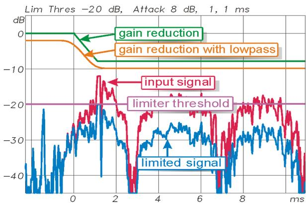
Figure 18: Limiter reaction to transient above threshold
