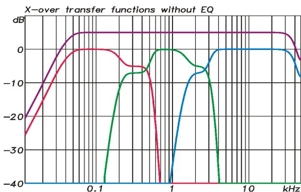
Figure 11: Resulting FIR filter and overall responses
