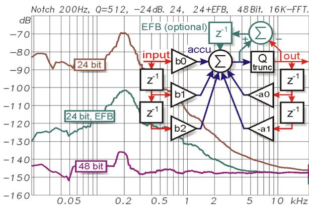
Figure 3: Topology of a biquad in direct form I with optional error feedback, and self-generated noise of a notch filter with single and double precision processing.
