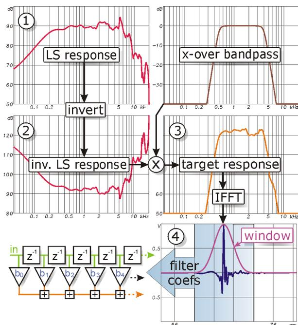
Figure 8: Simplified principle of complex EQ FIR filter coefficient generation for mid-range loudspeaker
