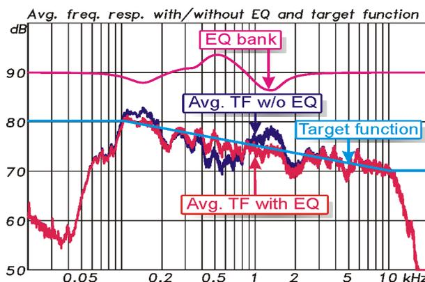
Figure 14: Averaged TFs without and with EQ, target response, and EQ curve
