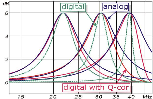
Figure 2: Transfer functions of analog and digital bell filters (6 dB gain,  $Q=4$ ), with and without  $Q$  correction
