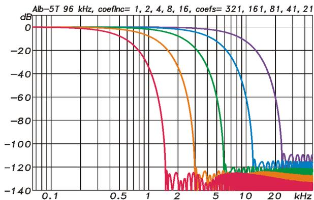
Figure 7: Frequency response of anti-alias low-pass for sample rate reduction factors of 2, 4, 8, 16 and 32
