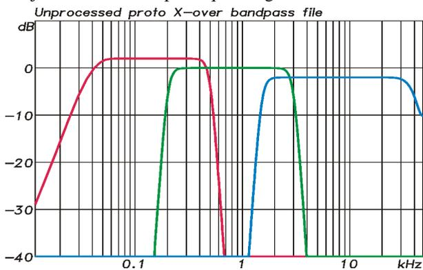
Figure 10: Example of overlapping prototype bandpass
