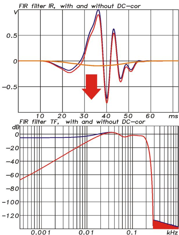
Figure 12: Original and DC-corrected filter IR and TF
