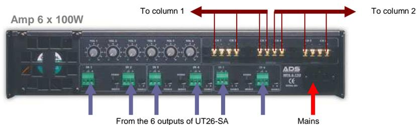
Figure 8 : Associating two 3 channel columns to a single 6 channel amplifier.
