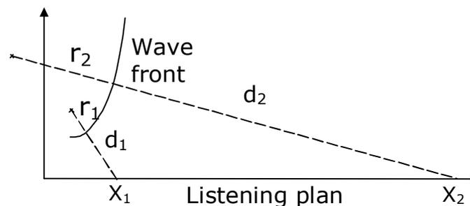
Figure 2 : *J* shape wave front required in order to radiate constant SPL over the listening plan.
