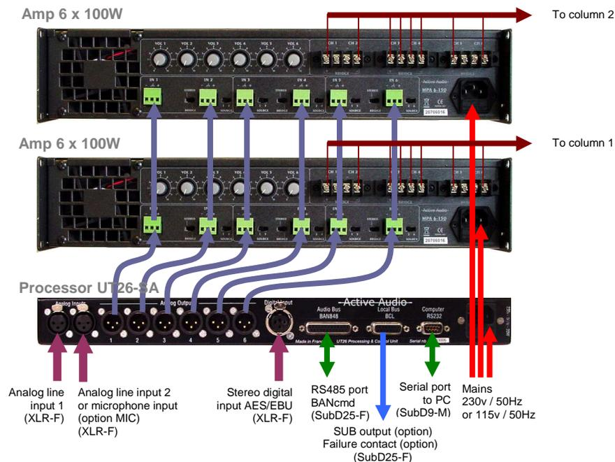
Figure 7 : Association of 2 amplifiers / columns to a single UT26-SA processor.
