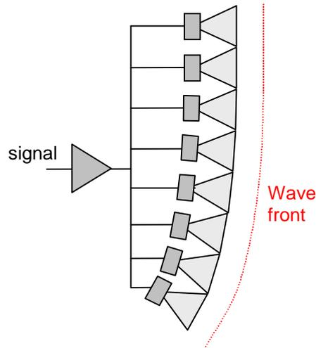
Figure 3 : In a geometric array, loudspeakers are aligned along the shape of the wave front to be generated, usually a J shape.
