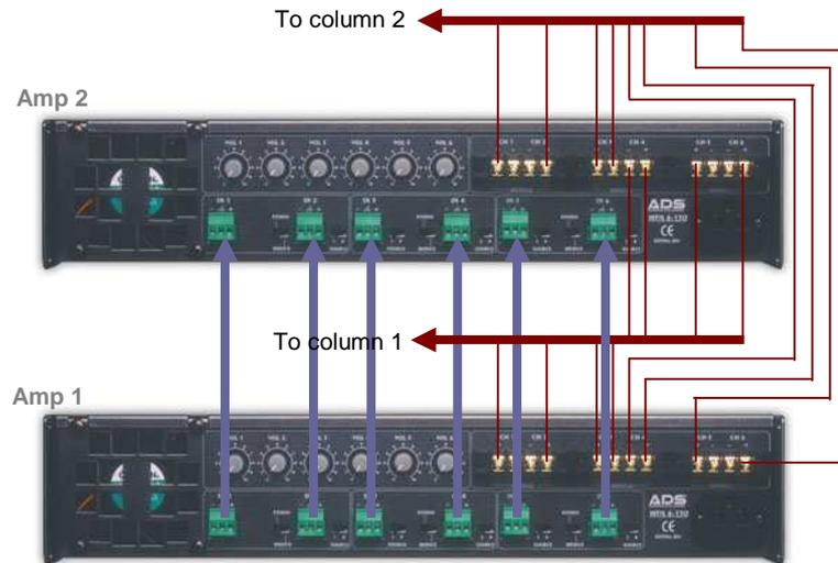
Figure 9 : Mixing the outputs of two amplifiers to two columns.
