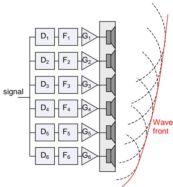
Figure 4 : In an electronic array, loudspeakers are aligned vertically, and the wave front is synthesized by adequate filtering by delays  $D_i$ , filters  $F_i$ , and gains  $G_i$  associated to each loudspeaker.
