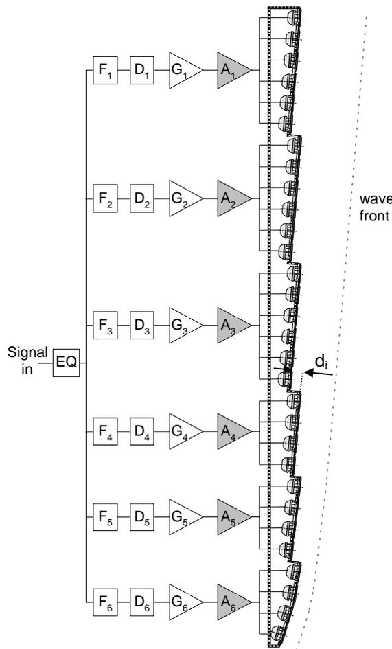
*Figure 5 : The DGRC principle used in StepArray columns. The wave front is controlled both by the positioning and orientations of the loudspeakers, and by the delays  $D_i$ , filters  $F_i$  and gains  $G_i$  of each channel.*
