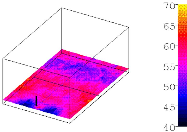
*Figure 6 : Example of RASTI modeling using software Catt®.
